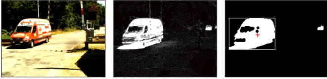
Figure 2. Example of centroid determination
