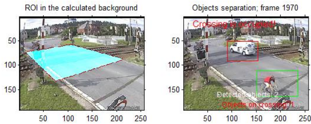
Figure 7. Objects separation over lower quality data
