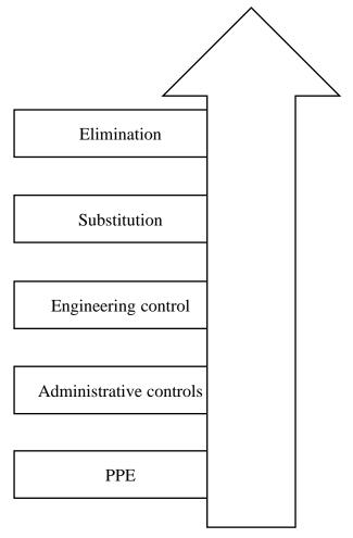
Figure 5. Hierarchy of controls [10]
