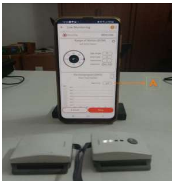
Fig. 12. Pheeze® EMG readings showing ambient noise of 1 uV (A) when no EMG source is connected
