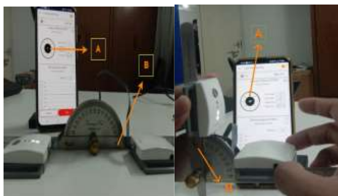
Fig. 9. Pheeze ® calibration verification tests with modules placed parallel: A) Pheeze app 0° B) goniometer 0° and perpendicular: A) Pheeze app 90° B) goniometer 90°.
