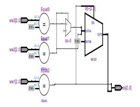
Figure 2 RTL View of Barrel Shifter
