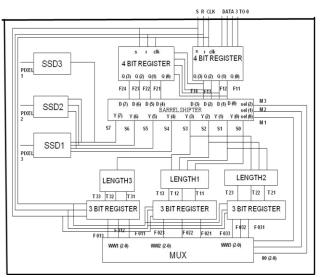
The Variable Length Decoder consists of 4-Bit Registers , Barrel Shifter , Seven Segment Display ,3 Bit Register and Multiplexer.
