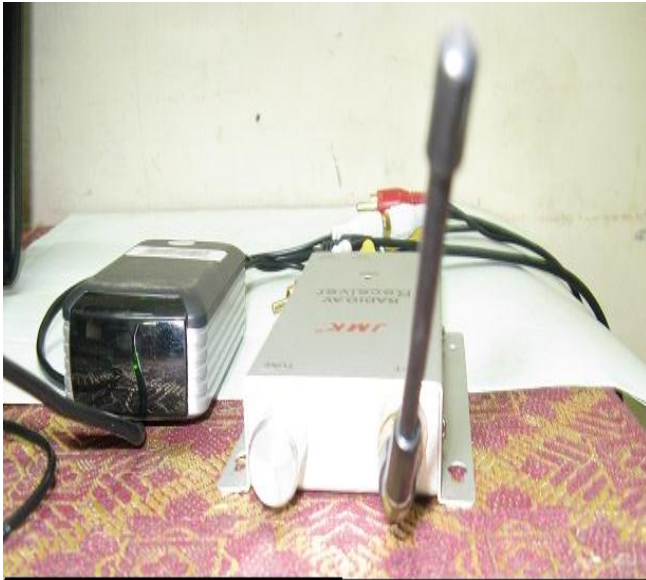
Fig. 8 Video receiver unit at control room
