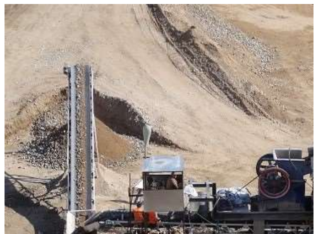
Figure 6: Crushing and sorting plant of C&D waste containing limestone in Gaza Strip (Photo by Yoshida, 2015)
