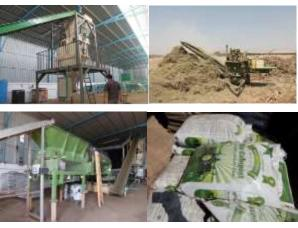
Figure 2: Production line, screening and packaging of compost product in PFC plant
