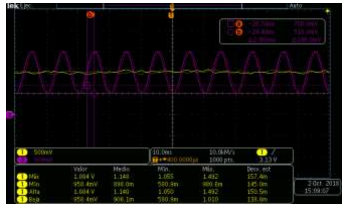
Figure 6. Measurements of e(n) and x(n) in the ANC system.
