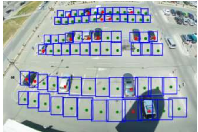
Fig. 7. A result when we do not classify with the optimal SVM model (there is an error on the second row from down/left)
