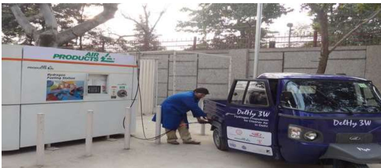
Figure 5 Hydrogen fuelled 3-wheeler developed jointly by IIT Delhi and Mahindra & Mahindra
