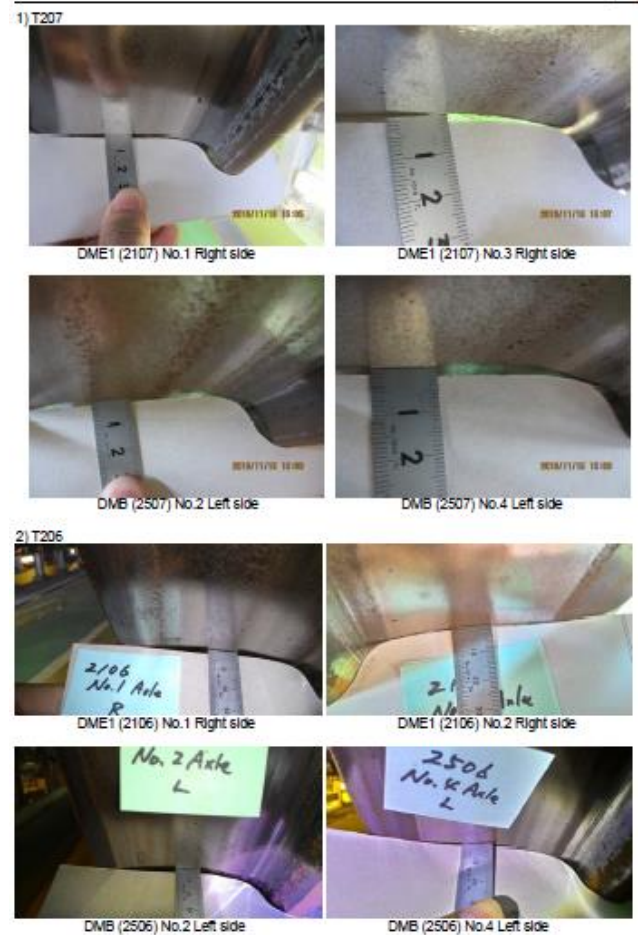
Figure 6: T206 and T207 steel wheel measurement
