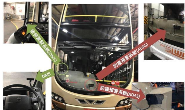
Figure 6a. The installation of DDDS and ADAS on board (Outside view)
