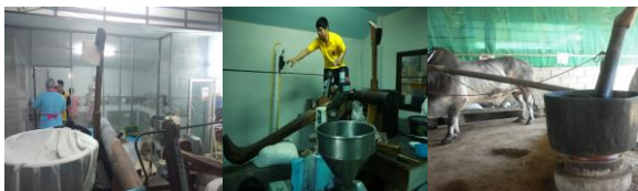
Figure 2 Sesame oil production by using mortar and pestle by cold extraction method of Ban Pang Moo Healthy Sesame Group Source: Research
