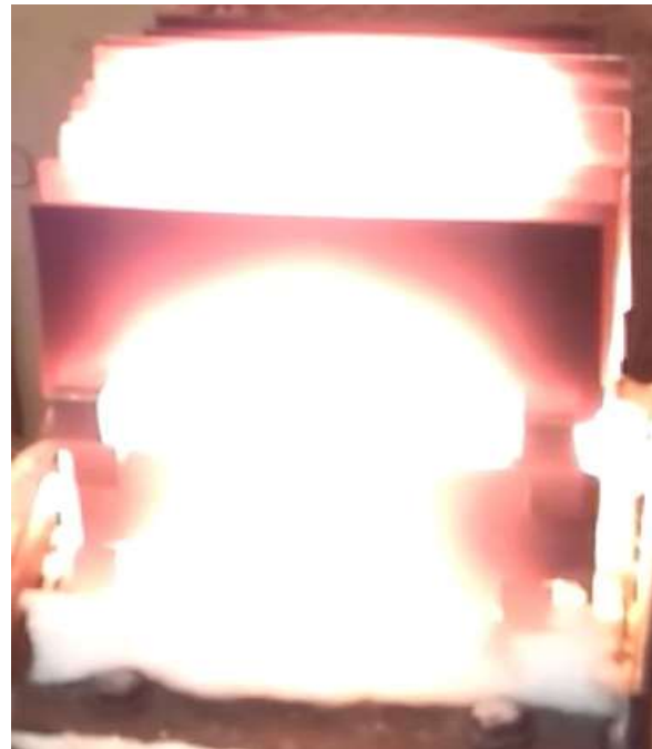
Figure 1. Photo of a laboratory layout of an IR burner operating without a fine-pored matrix. Power 16 kW, flow cross-section area 30 \text{ cm}^2 . The concentration of nitrogen oxides in the combustion products is 14 ppm, the concentration of carbon monoxide is 20 ppm with a value of air ratio 1.4. The maximum surface temperature of the recuperative elements is 1450^\circ\text{C} .
