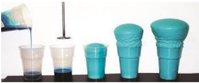
Figure 2: The steps of preparing the polyurethane compounds.
