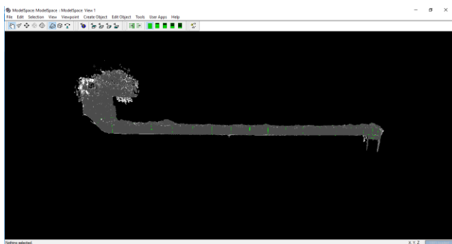
Figure 3.- Elevation view of the tunnel in Leica Cyclone.
