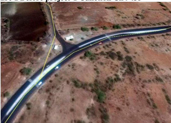
Figure 2 After project T-Junction with right turning lane Ch 9435
