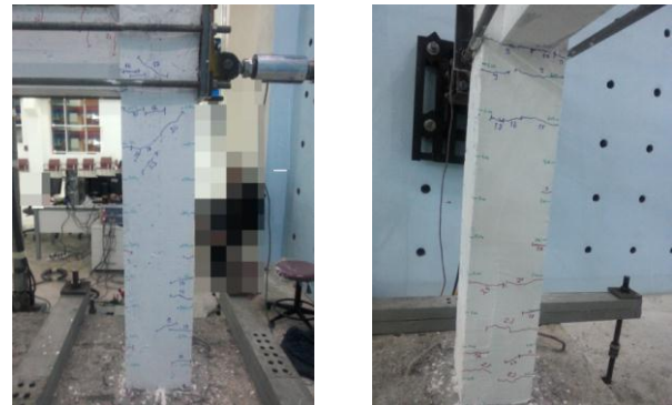
Fig. 9: CBFS-D Specimen's Crack Development
