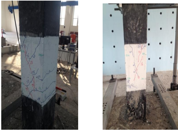
Fig. 10: CBFS-DC Specimen's Crack Development
