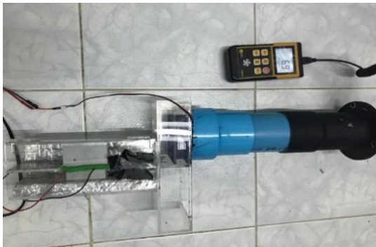
Figure 4. Air measurement while vary the fan voltage supply
