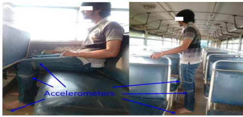
Figure 3.0 Placement of accelerometers under sitting and standing orientations of the passenger
