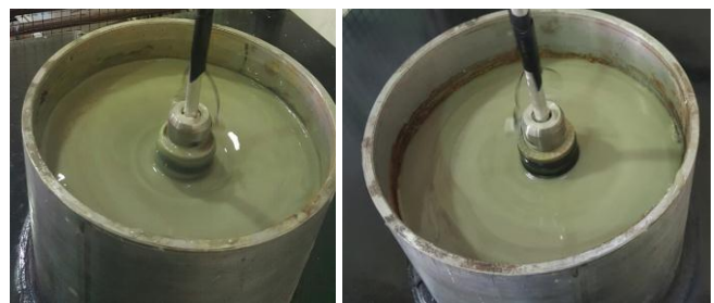
Figure 7. Experimental observation of rotor motions illustrating system behavior at (1) low ( \Omega=5.23(2\pi) rad/s) and high ( 10.47(2\pi) rad/s)
