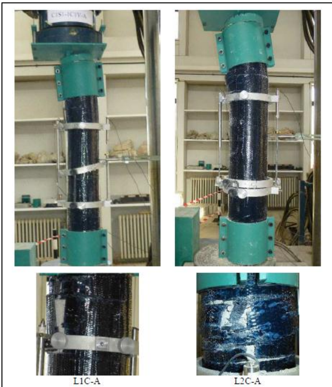
Figure 4. Examples of failure patterns of FRP-jacketed columns
