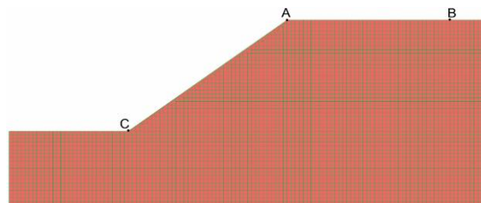
Figure 3. Geometry C: Discrimination of slope geometry with 4:3 slope.
