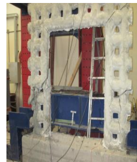
Figure 11 SD2 after applying cyclic load
