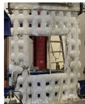
Figure 5 SW2 after cyclic loading
