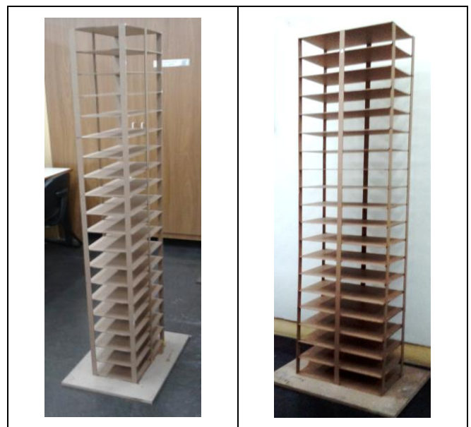
Figure 1. Investigated 19 story HDF building constructed in laboratory.
