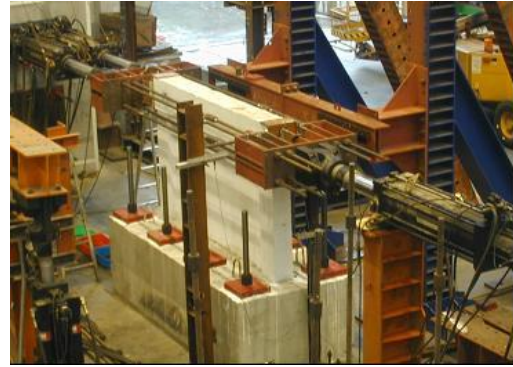
Figure 5. Set-up of reversed cyclic tests
