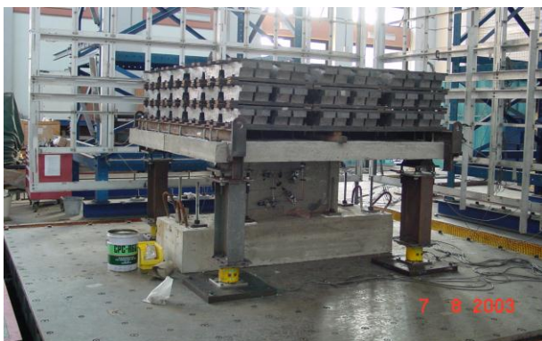
Figure 2. Test set-up of shake table tests
