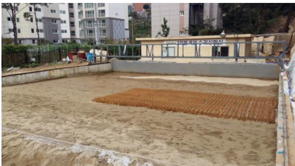
Figure 2. Model beach of installing with the Coral cell or without Coral cell
