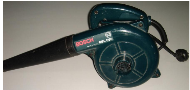
Figure 6. The blower used to clean the dust.
