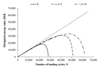
Figure 3. Evolution of DER as a function of loading cycles for blends with increasing crumb rubber dosage (example)
