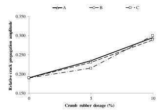
Figure 4. Variation of the RCPA parameter as a function of crumb rubber dosage for the considered blends
