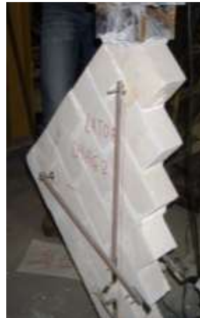
Figure 16. Resulting pieces after diagonal test
