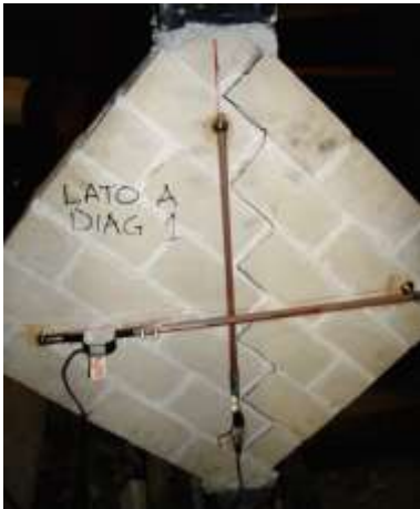
Figure 15. Cracks after diagonal test
