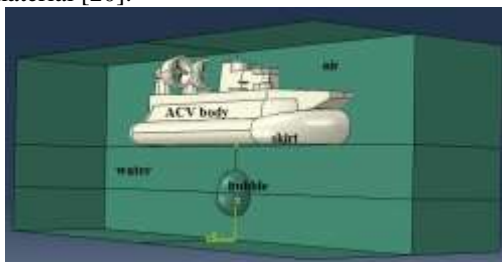
Figure 7. Set up model of ACV's skirt response The mechanical properties of the hovercraft body and especially skirt properties are shown in TABLE 3.
