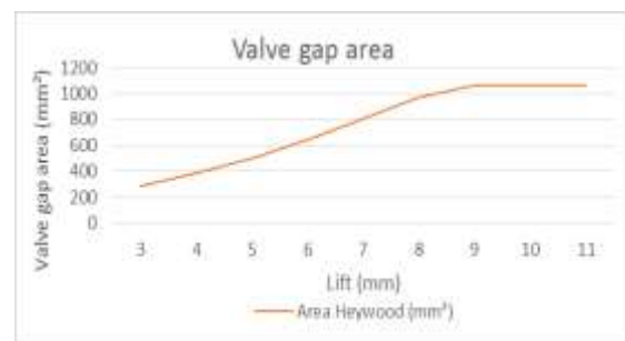
Figure 14: Valve gap area
