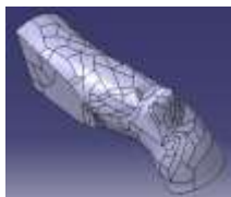
Figure 4. IGES exhaust conduct
