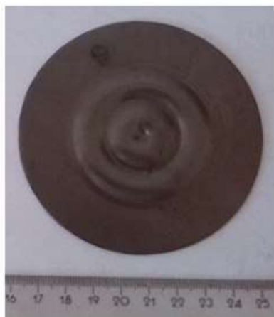
Figure 4. Part obtained by One-channel sheet hydroforming
