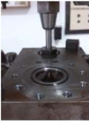
Figure 2. View of the hydroforming die
