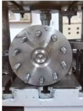
Figure 3. Upper plate of the die with active zone and screws
