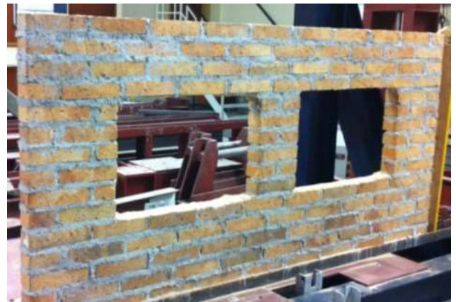
Figure 1d Wall with 30% opening
