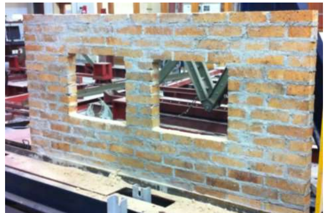
Figure 1c Wall with 20% opening
