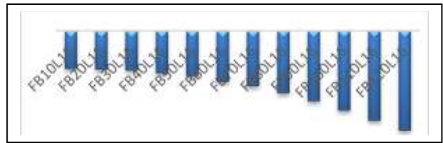
Figure 6(b). Minimum wavelet coefficient for continuous wavelet transform for cracks at L/16 location with a varying crack depth.
