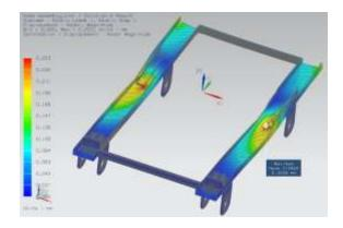
Figure 9. Maximum Displacement of 0.253 mm for Base Structure Assmebly
