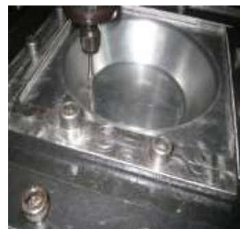
Figure 5: A model of SPIF is being machined in specified features in SPIF machine.
