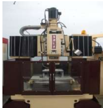
Figure 4: SPIF machine and feature in forming Titanium sheet, selected sheet thickness is 1mm
