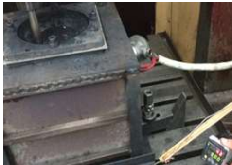
Figure 7: Heating system under SPIF feature 3
