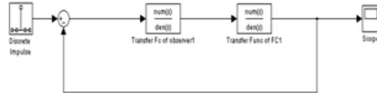
Figure 8 . Simulink circuit of the model of fuel cell system in closed loop configuration with minimum order observer.
