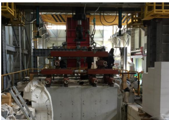
Figure 4. Specimen in a furnace
