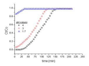
**Fig. 5.** Experimental breakthrough curves of Fe<sup>+3</sup> as a function of pH of solution (T 15°C, bed depth 5 cm, Co 50 ppm, flow rate 5 mL.min<sup>-1</sup>, particle size 0.25-0.5 mm).
