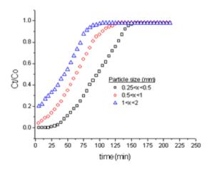
**Fig. 6.** Experimental breakthrough curves of Fe<sup>+3</sup> as a function of particle size (T 15°C, bed depth 5 cm, Co 50 ppm, flow rate 5 mL.min<sup>-1</sup>, pH 4).
