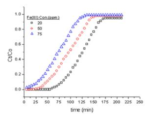
**Fig 1.** Experimental breakthrough curves of Fe<sup>+3</sup> as a function of inlet Fe<sup>+3</sup> concentration (T 15°C, pH 4, flow rate 5 mL.min<sup>-1</sup>, bed depth 5cm, particle size 0.25-0.5 mm)
