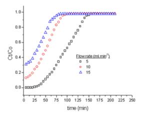
**Fig 2.** Experimental breakthrough curves of Fe<sup>+3</sup> as a function of flow rate (T 15°C, pH 4, Co 50 ppm, bed depth 5 cm, particle size 0.25-0.5 mm).
