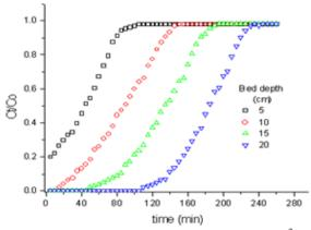
**Fig 3.** Experimental breakthrough curves of Fe<sup>+3</sup> as a function of bed depth (T 15°C, pH 4, Co 50 ppm, flow rate 5 mL.min<sup>-1</sup>, particle size 1-2 mm).
