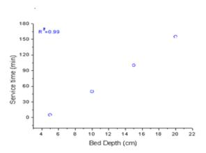
**Fig 4.** BDST model (Co 50 ppm, pH 4, flow rate 5 mL.min<sup>-1</sup>).
