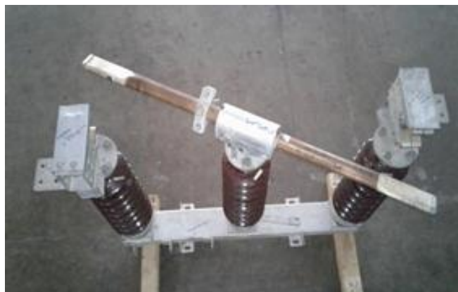
Fig. 2 A View of Movable assembly for 66 kV Isolator
