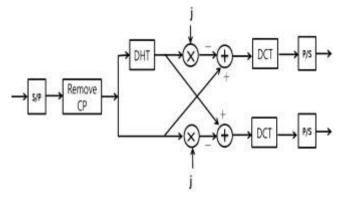
Fig.2. Receiver of proposed OFDM-SSB system.
