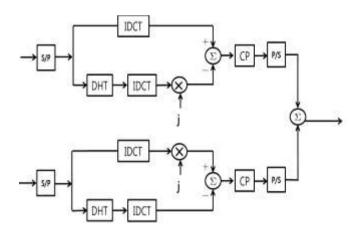
Fig.1. Transmitter of proposed OFDM-SSB system.
