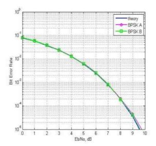
Fig. 5. BER performance of BPSK OFDM-SSB in AWGN.
