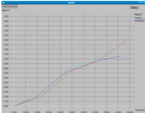
Figure 5. Delay in DSDV,AODV and QOSUNIFIED
