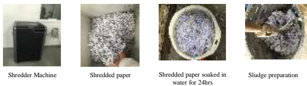
Figure 1. Sludge preparation from waste papers
