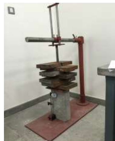
Figure 5. Experimental set up for creep test
