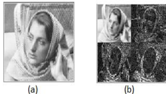
Figure 1. Figure showing (a) The original woman image (b) The 2-D wavelet decomposed representation of the woman image. The bands are labeled as LL1,HL1,LH1,HH1 following from top-left to bottom-right. The LL1 sub-band contains the most significant image coefficients, while HL1, LH1 and HH1 sub-bands contain only the directional information.
