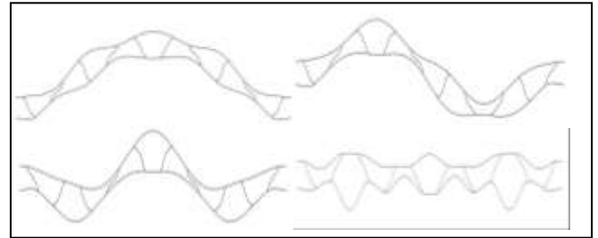
Figure 2. From top left: first three modes of vibration. In the bottom right corner an example of local mode for 1887 Hz.
