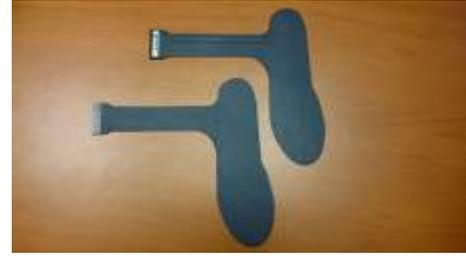
Figure 1. Instrumented insoles.
