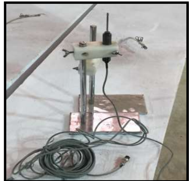
Figure (5) LVDT to measure the deflection
