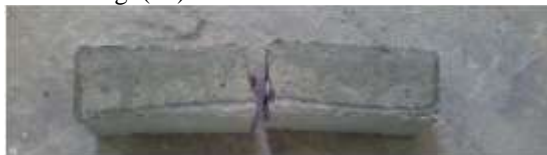
Figure 16. Fracture Shape (Brittle Failure) of PC Beam.
