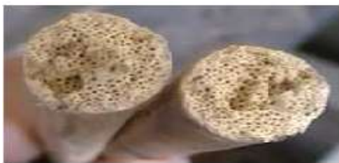
Figure 3. Brittle shape of failure.
